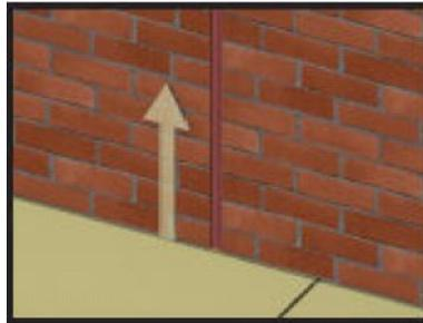
5. Run a 1/4" bead of the supplied silicone adhesive along both joint walls approx. 1/2" – 3/4" back from the surface of the joint substrate.
