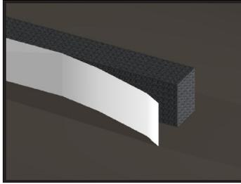
5. Place the material into the joint while gently pushing the pressure sensitive adhesive (PSA) up against the side of the substrate. Once the material is in place, use a margin trowel to firmly press the adhesive to the substrate and allow the material to expand to fill the joint.
