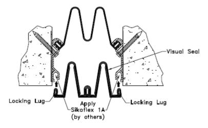
6. Before installing visual seal, apply Sikaflex 1A adhesive into front locking cavities of aluminum extrusions. Ensure full engagement of locking lug.
