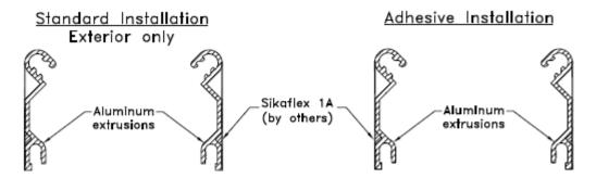
1. Apply adhesive along back of the aluminum extrusions prior to installation—following adhesive manufacturers guidelines.
