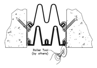
7. Utilizing roller tool, apply pressure directly over locking lug to ensure proper engagement of seal lug.
