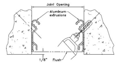
3. Position aluminum extrusions and mark hole locations. Drill holes through aluminum flange and into wall for 3/16" Tapcon screws @ 18" O.C.
