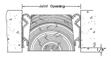
2. Field measure all lengths and directional changes for aluminum extrusions to ensure their proper layout where required. Mount extrusions to wall surface and install temporary wood blocking to secure extrusions to wall while adhesive cures and for field drilling for standard installation. Wood blocking should be non-continuous to permit field drilling of anchor holes at required spacing. Contact adhesive manufacturer for proper cure times before proceeding to next step.
