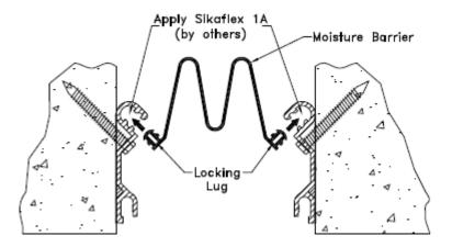
5. Before installing moisture barrier, apply Sikaflex 1A adhesive to rear locking cavities of the aluminum extrusions. Ensure full engagement of locking lug.
