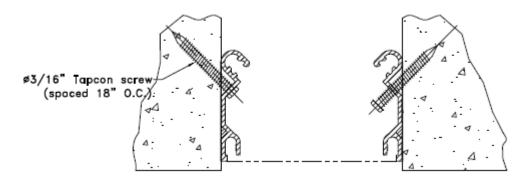
4. Secure aluminum extrusions to wall with 3/16" Tapcon screws @ 18" O.C.
