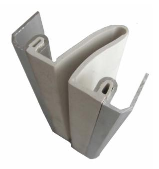
The Seismic Elastomeric Ceiling System uses an aluminum channel attached to the grid system above the sight line. The finished Santoprene seal comes in four colors to match your surrounding substrate and finish material. This system accommodates seismic movement.
