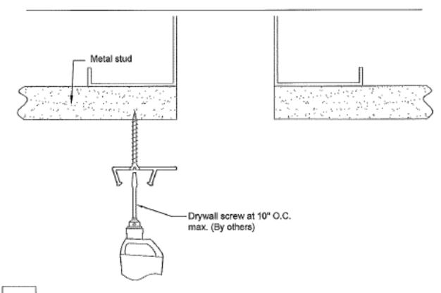
Align and drive drywall screw through base extrusion into wall construction at the specified anchor spacing.
