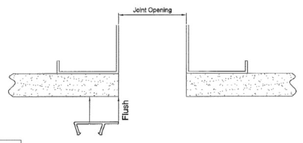
Position base extrusion onto wall flush with edge of joint opening.
