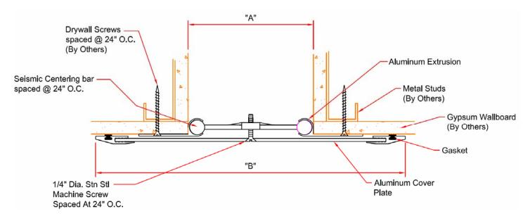
EFCT-400 THRU EFCT-2400 DETAIL WALL TO WALL OR CEILING TO CEILING INTERIOR CONDITION
