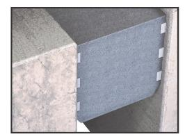
**CONTACT EMS FOR PROPER SIZING - Supplied** material should be approx. 25% larger than the intended joint opening.
