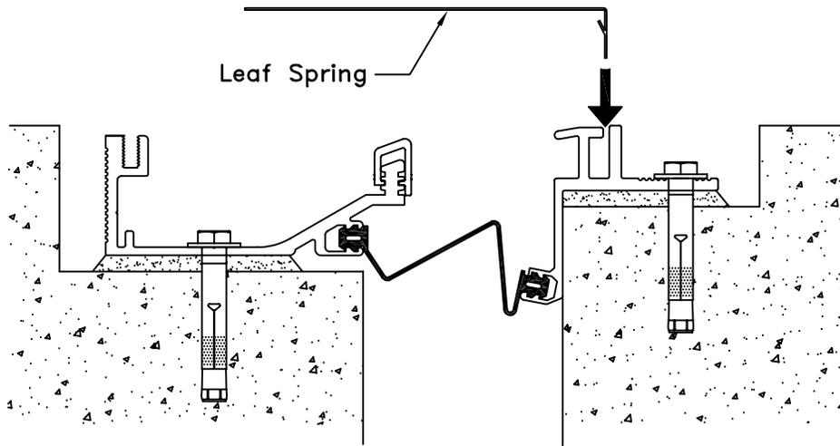
**7** Snap leaf spring into leaf mount extrusion. Ensure top surface of leaf mount extrusion is flush with top surface of leaf spring.
