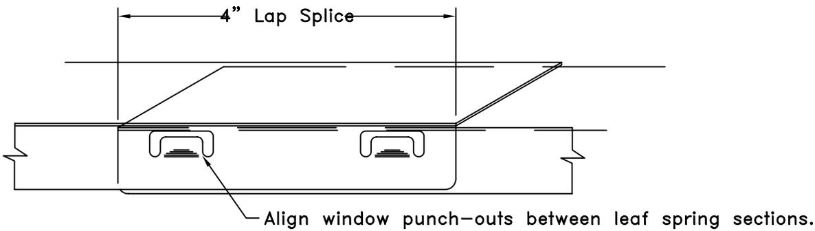
**8** Stagger all splices in accordance with detail illustrated above to provide a stronger assembly and durable installation.
