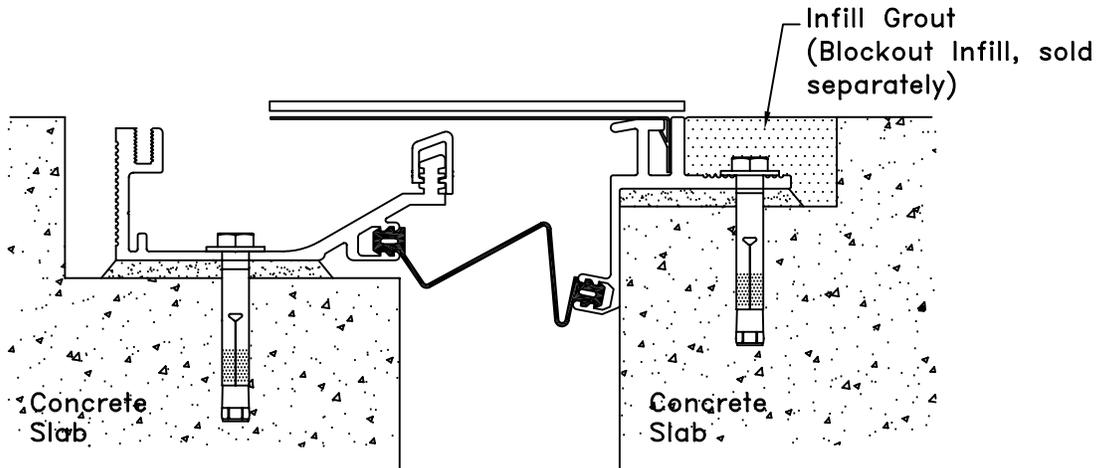
**9** Install Grout into blockout on Leaf Spring Side after Leaf Spring and anchors have been installed.
