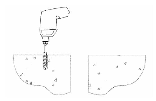
2. Drill end holes first, this ensures the cover plate will not move and alignment with other joints is obtained. Cover plates are supplied with predrilled holes, using a 1/4" concrete drill bit drill holes to a depth of 2-1/2".
