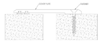
1. Cut and fit cover plate to required length, if installing more than one piece, lay out entire run to ensure proper alignment. Make sure that the pre-drilled holes are lined up at least 1-1/2" from the edge of the expansion joint.
