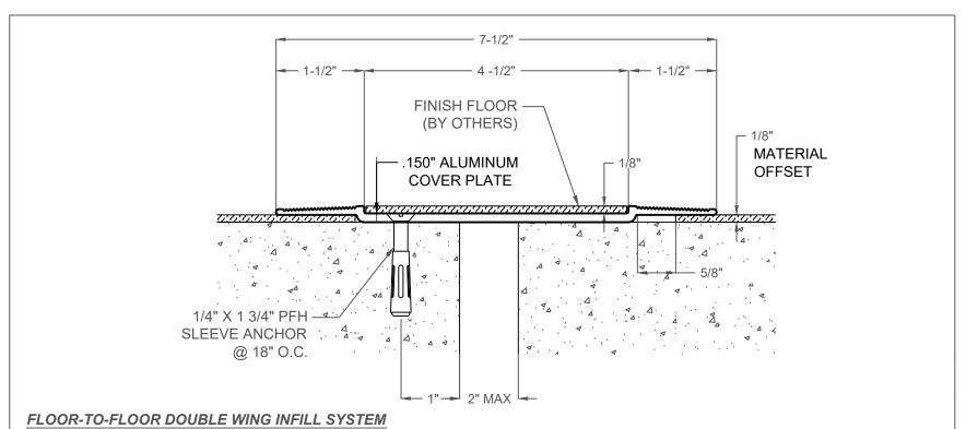
EXPOSED FINISH: MILL MOVEMENT: +/- 5/8" STOCK LENGTHS: 10'-0"
