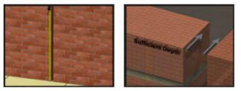
**NOTE:** Allow sufficient depth for the material to be recessed 1/8"- 1/4" in the joint.
