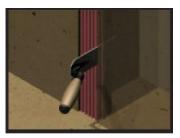
7. Silicone coating should be flush with, not protruding above, the substrate surface.
