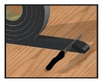
3. If the joint runs horizontal, begin installing the material at one side of the joint (either side) and continue to install the material working towards the opposite end. For vertical joints begin installation at the bottom of the joint and work upward.
