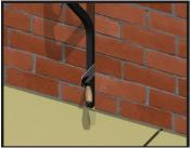
**WARNING:** Allow 72 hours for full expansion and material equalization. Expansion and equalization rates are affected by temperature. Material will expand faster when hot and slower when cold.
