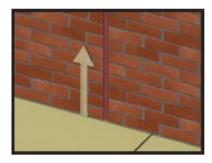
5. Run a  $\frac{1}{4}$ " bead of the supplied silicone adhesive along both joint walls approx.  $\frac{1}{2}$ " -  $\frac{3}{4}$ " back from the surface of the joint substrate.
