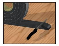
3. If the joint runs horizontal, begin installing the material at one side of the joint (either side) and continue to install the material working towards the opposite end. For vertical joints begin installation at the bottom of the joint and work upward.
