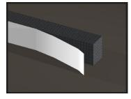
5. Place the material into the joint while gently pushing the pressure sensitive adhesive (PSA) up against the side of the substrate. Once the material is in place, use a margin trowel to firmly press the adhesive to the substrate and allow the material to expand to fill the joint.
