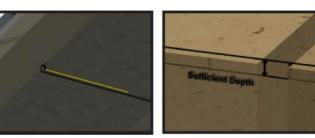
**NOTE:** Allow sufficient depth for the material to be recessed 1/8"– 1/4" in the joint.
